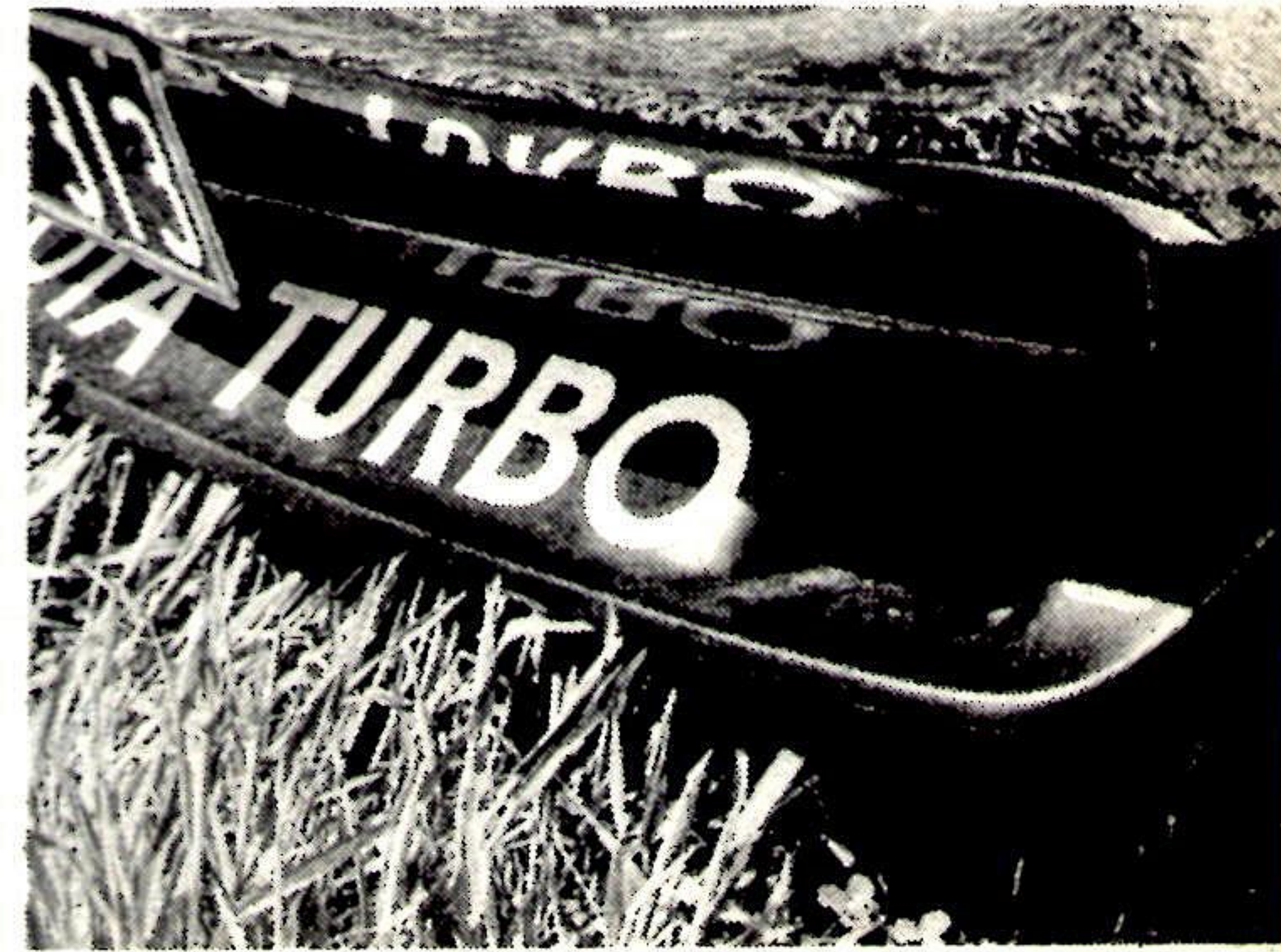
RIGHT: The signwriting was a bit much for us, but the spoiler and its brake-cooling air scoops worked well. LEFT: Cooling air is fed back to the brakes through this fibreglass tube, an extension of the spoiler. A 'rest' of a few hundred metres was enough to allow the fading brakes to cool — so the air ducts do their job.
